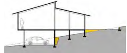
Where slabs are used on slopes between 7% and 20%, they should step down the hillside.
